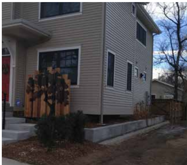
Floodplain requirements often result in new construction that is raised or elevated above base flood elevations, which may interrupt the established character of a block as new construction "sits" higher than adjacent homes.
